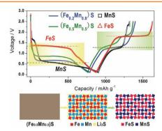
A series of  $Fe_xMn_{1-x}S$  (x = 0.2, 0.5, 0.8) monosulphide compounds is synthesized using a simple solid state reaction method. The lithium storage voltage can be tuned by the content of Fe in Fe<sub>x</sub>Mn<sub>1-x</sub>S, while the electrochemical performance of electrodes based on  $Fe_xMn_{1-x}S$  is greatly enhanced in comparison with that of MnS. The lithium storage mechanism of  $Fe_{0.5}Mn_{0.5}S$  is investigated in detail.
