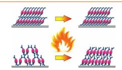
Substituting a dicyanoperylene molecule with asymmetric branched alkyl chains is revealed to be an effective strategy for obtaining, upon thermal annealing, fieldeffect transistors with enhanced transport properties with respect to linear alkyl chains.
