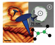
The structure, energy and topology of ferroelectric domains pinning as a result of extended structural defect are studied. Enhanced piezoresponse force microscopy is used to study the statics and dynamics of pinned domains. The pinning is analyzed in terms of Bornarel's theory, and Srolovitz and Scott's model, while a quantitative method to evaluate the energy of a pinned or distorted domain using the Landauer framework is presented.
